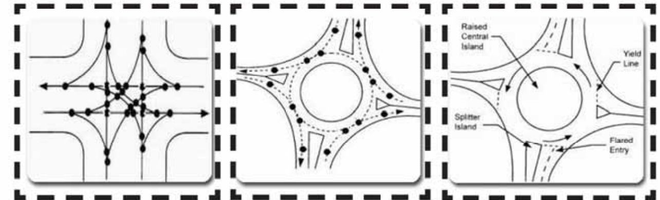
Image 1 indicates the 32 conflict points a traditional intersection has.
