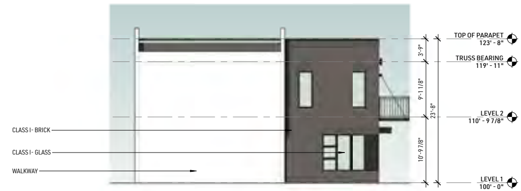
EXTERIOR ELEVATION G
