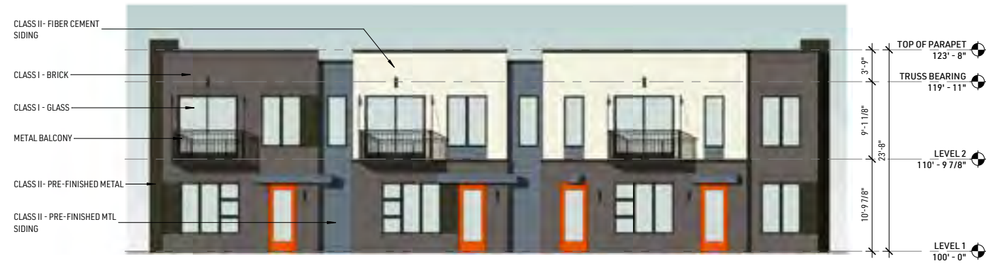
EXTERIOR ELEVATION B
