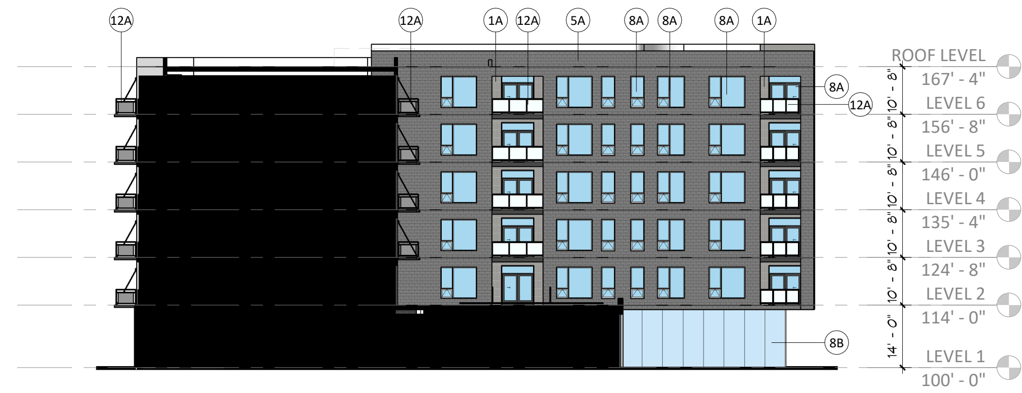
6 WEST ELEVATION - COURTYARD - COLOR A3-0 3/64" = 1'-0"
