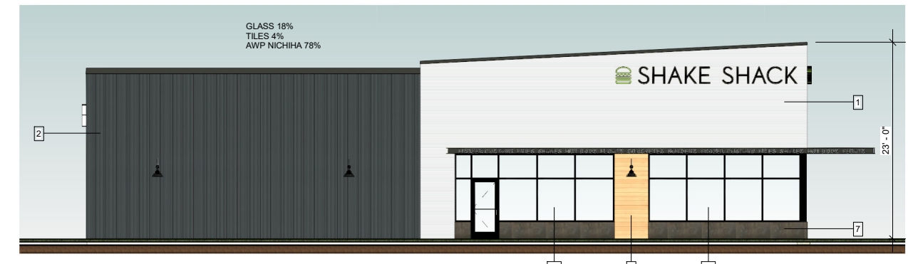
6 EAST ELEVATION - SHAKE SHACK 1/16" = 1'-0"
